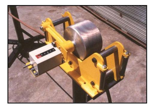
The MU100 is used for the accurate measurement of cable, rope, hose, etc, from 2mm outside diameter up to 100mm. The alluminium measuring wheel is directly connected to the re-settable counter and spring loaded to ensure good contact between wheel and cable. The meter can be bench mounted or fitted to a fabricated stand to give a convenient operating height.
